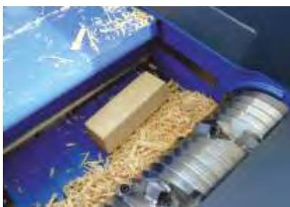
Rotor with one row of knives for low power consumption
