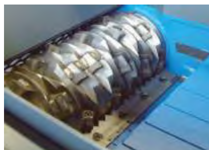
Rotor with a diameter of 368 mm with two rows of knives for higher throughput
