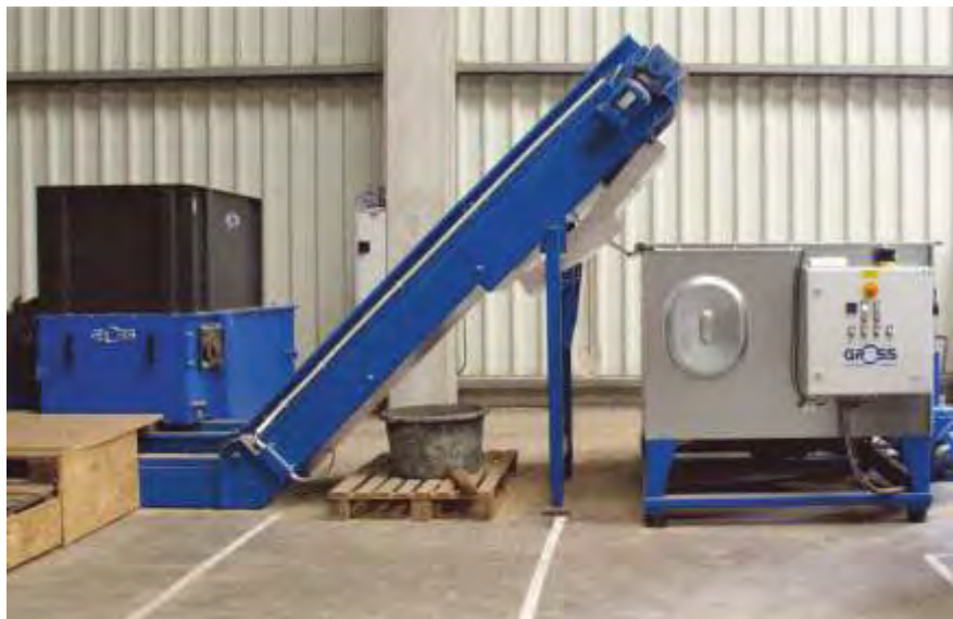
GAZ 82 S in combination with conveyor belt and briquetting press
