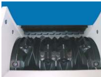
Rotor, Ø 368 mm
